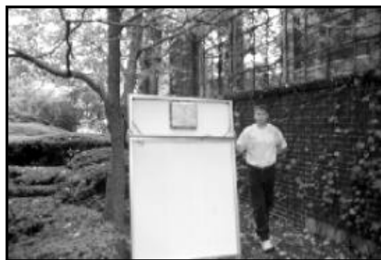
Figure 1: Back of Ascension Technology's "SunSine300™ AC Module " illustrating the AC inverter.
