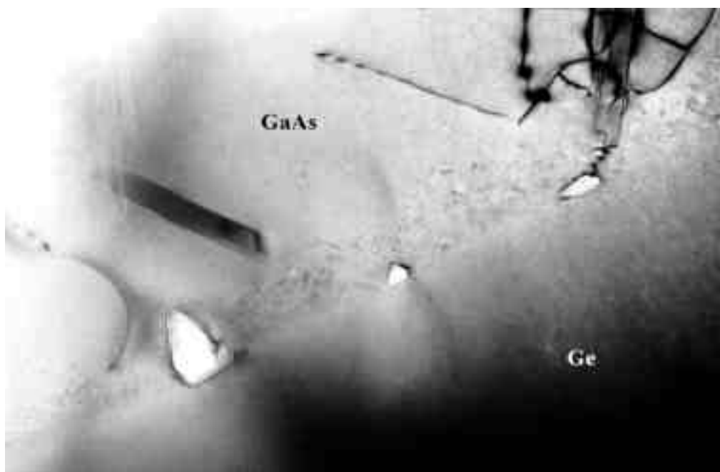
Figure 8. TEM micrograph showing antiphase domains (small truncated triangles) at the GaAs/Ge interface. The Ge(100)6°(111) substrate was annealed in AsH 3 under conditions similar to those used in Fig. 5.
