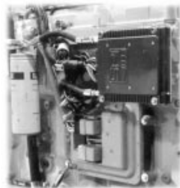
Dual-fuel electronic control unit (ECU) controls air/fuel ratio, fuel quality and injection timing.
