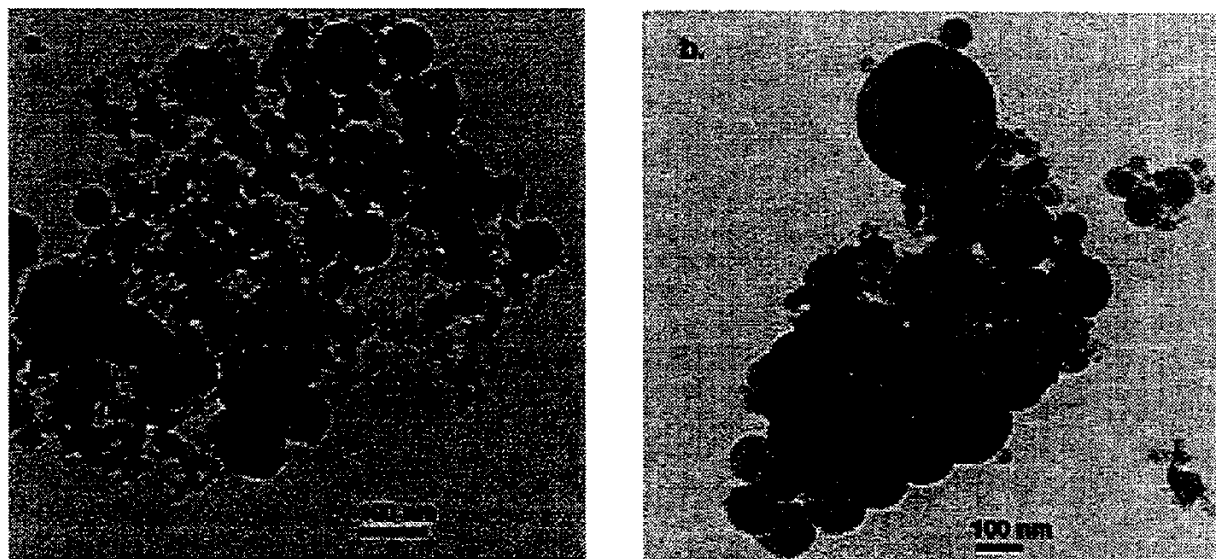
Figure 1. TEM micrographs of nano-Al prepared by electroexplosion method.
