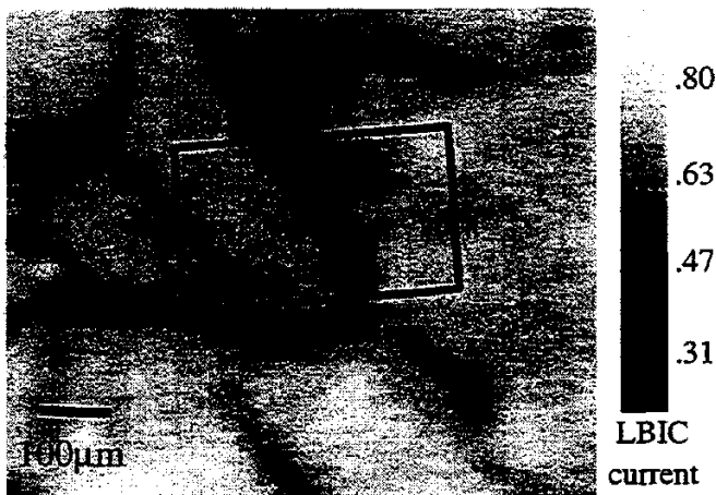
Figure 1: Light Beam Induced Current map of carrier recombination across a portion of multicrystalline silicon. Dark regions indicate high carrier recombination. The black box denotes the area analyzed with x-ray fluorescence.
