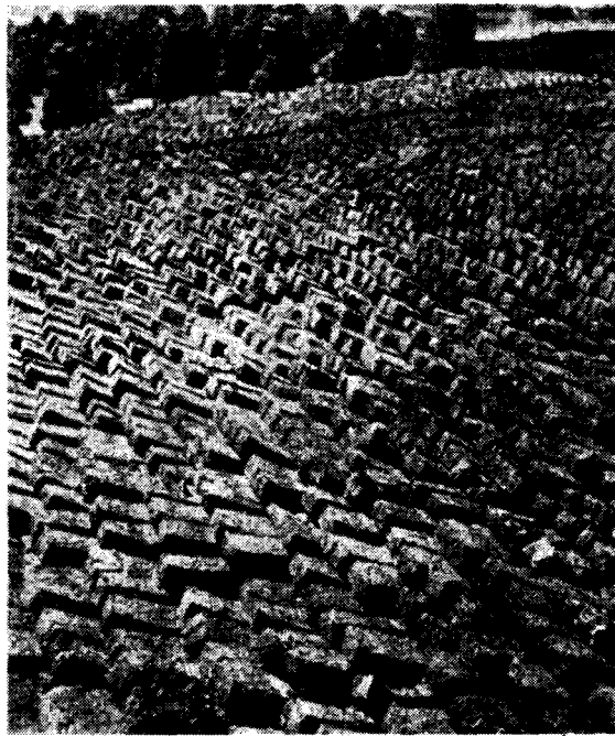
Figure 56. Sun-drying of peat. (Peat stacks in the background)
