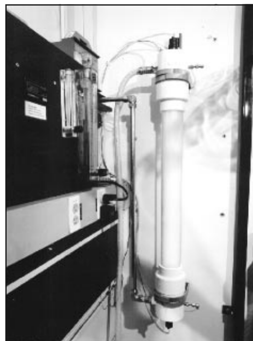
(Above) IT Corporation's pilot-scale detoxification system. Researchers use this portable unit at waste sites to determine if detoxification technologies can be successfully applied given the site-specific conditions. (Right) A laboratory-scale version of IT's gas-phase detoxification reactor. SI program researchers continue to improve process performance in the laboratory. The TiO 2 catalyst suspended in the reactor vessel can be activated by either sunlight or electric ultraviolet light.
