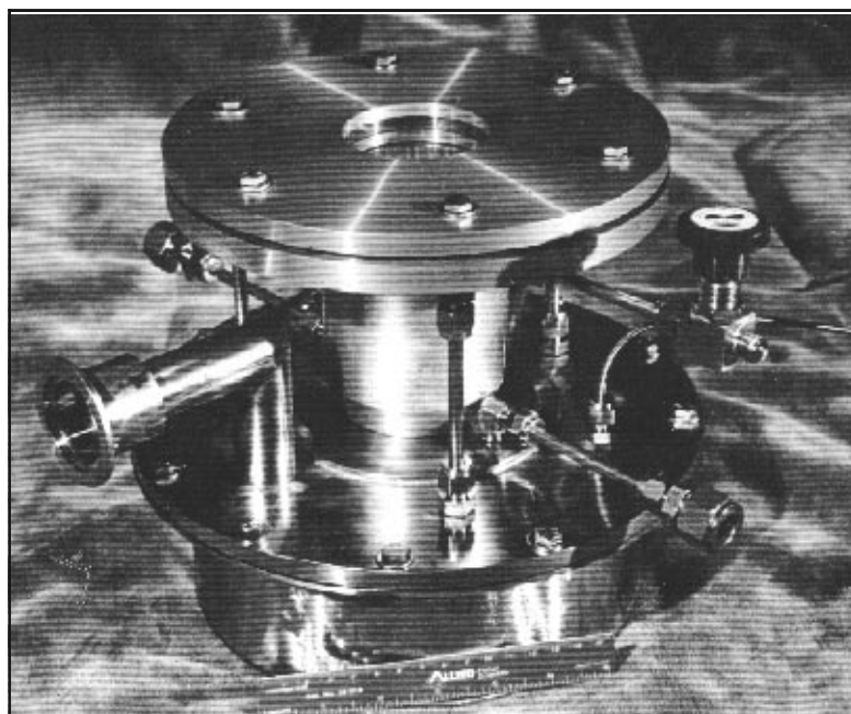
Fullerene reaction chamber. Researchers at the National Renewable Energy Laboratory used this device to synthesize fullerene molecules by bombarding a graphite pellet with solar flux. A turning mirror (not shown) mounted above the chamber directed concentrated solar flux produced by the HFSF into the aperture in the center of the top plate, shown here.
