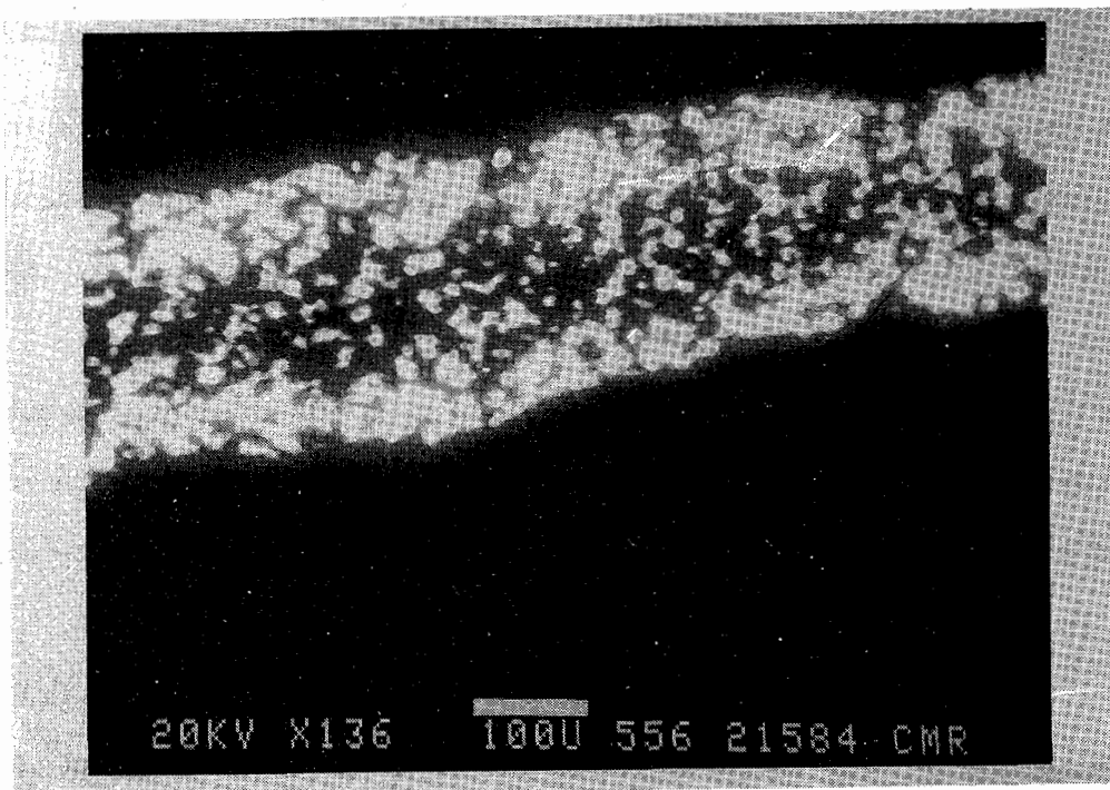
Fig. 7. EBIC scan of a CdS/CdTe/graphite cell with a very thin CdS layer (2 layers of 300 Å each) (magnification 136X). The CdS coverage appears to be discontinuous and collection occurs only around the In contact strip. (Positive image: light areas show greatest collection).
