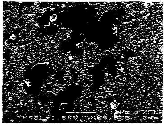
Figure 1: SEM micrograph of a 40-nm thick CdS Film, showing gross discontinuities and pinholes.
