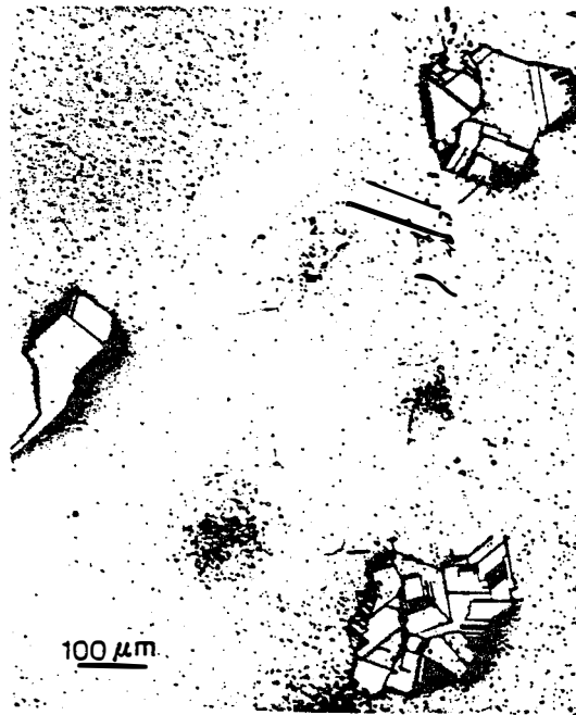
Fig. 9. A light micrograph of an area of twin-stabilized growth in a LASS sample illustrating localized defect structures.
