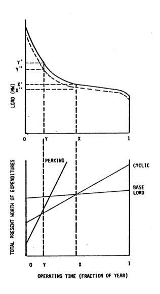
Screening Curve Approach to Determine Optimal Generation Mix
