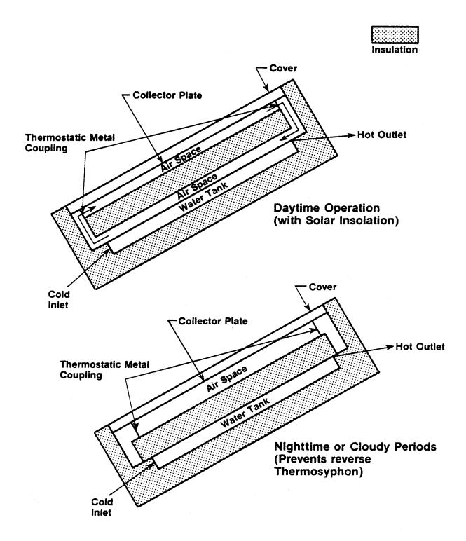
Figure 3-1. Schematic of Thermosiphon Concept
