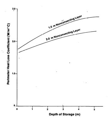
Figure 5-2. Perimeter Heat Loss Coefficient of Salt Gradient Pond as a Function of the Nonconvecting and Storage Layer Depths
