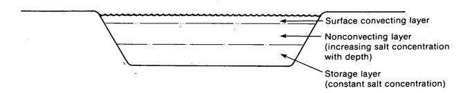
Figure 2-1. Salt Gradient Solar Pond
