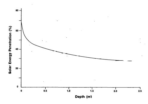
Figure 5-1. Optical Transmission  $\overline{\tau\alpha}$  as a Function of the Depth of the Surface-Convecting and Nonconvecting Layers Combined
