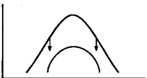
Figure P-5. Typical load shape changes resulting from selected demand-side alternatives. Adapted from Clark W. Gellings, highlights of a speech presented to the 1982 Executive Symposium of EEI Customer Service and Marketing Personnel.
