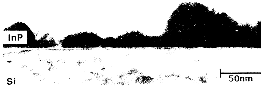
Figure 3.3: The three-dimensional nucleation of InP on Si.
