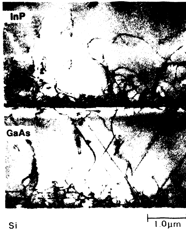
Figure 3.6: TEM cross section showing the deterioration of InP under thermal annealing.
