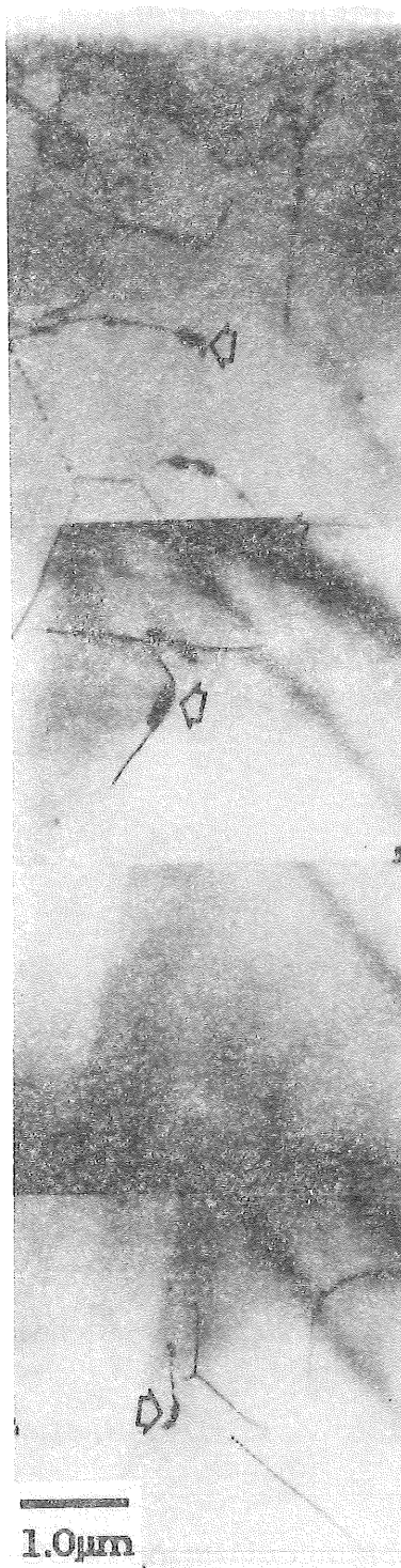
Figure 3.18: [112] cross section showing a heavily damaged region near the implanted surface and hydrogen decoration of dislocations deep in the Si (arrows).
