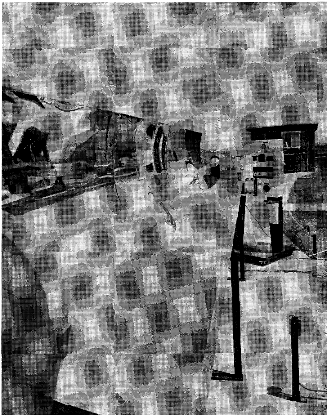
Figure 1. Experimental Solar Decontamination Trough.
