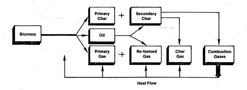
Figure 2. HEAT AND MASS FLOWS IN PYROLYSIS AND GASIFICATION PROCESSES
