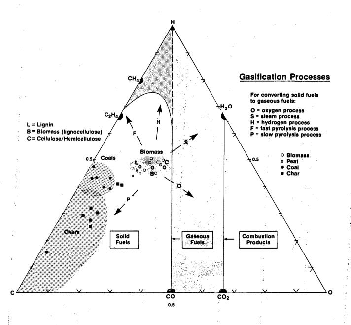
Figure 1. CHEMICAL CHANGES DURING BIOMASS GASIFICATION
