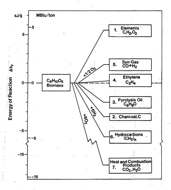
Figure 3. ENERGY CHANGES IN CELLULOSE THERMAL CONVERSION REACTIONS
