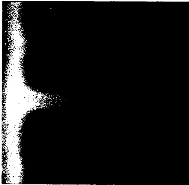
Fig. 6 - Plan view EBIC/SEM image, taken at room temperature, showing an individual dislocation diode with a dark recombination line in the center.
