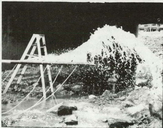
Figure 3-1b. High Flow Rate from a Slotted Pipe with 5 Slots Exposed, A_L = 3.0 , 13.8 kg/s Total Flow (Slots Pointed Upward)
