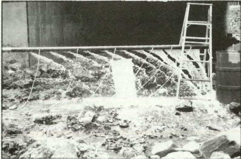
Figure 3-5a. High Flow Rate from a Slotted Pipe with 10 Slots Exposed, A_L = 6.0 , 13.7 kg/s Total Flow (Slots Pointed Downward)
