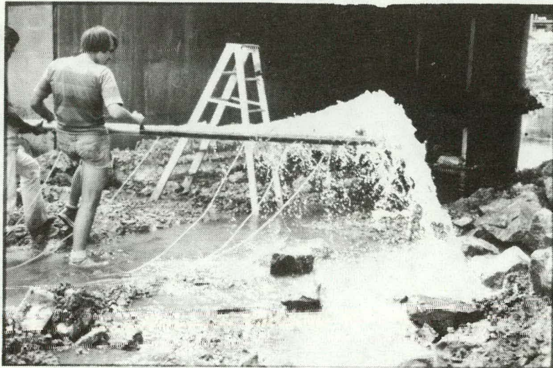
Figure 3-2a. Low Flow Rate from a Slotted Pipe with 5 Slots Exposed, A_L = 3.0 , 5.9 kg/s Total Flow (Slots Pointed Upward)
