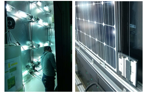
Fig. 2: The module hot spot test uses HQI lamps which generate 700 W/m 2 and a temperature of approx. 65 °C on module backside surface. For first test each cell is completely shaded for 15s (module is short-circuited). Backsheet temperature is monitored with an IR camera.
